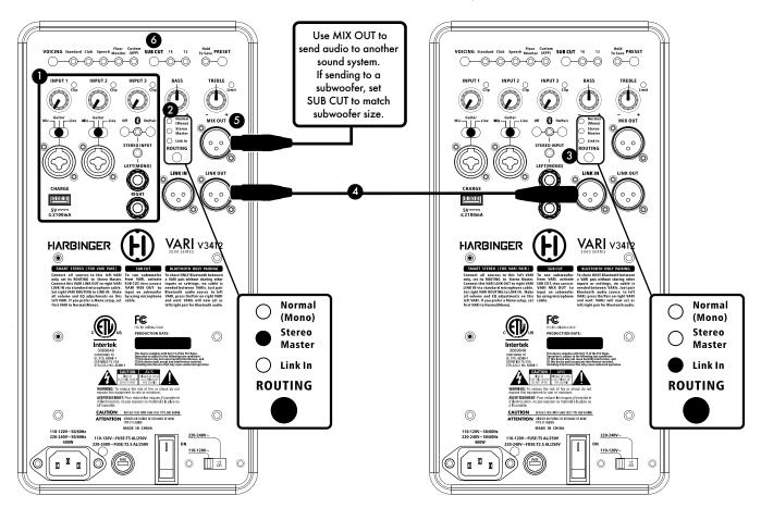
A pair of VARI V3412 or V3415 speakers can operate together as a Smart Stereo system, giving you control of the sound and volume of both speakers from the first master speaker, and optimally distributing all audio inputs to both speakers for rich stereo sound.
