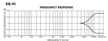
The high EQ control is a shelving EQ. What this means is that it boosts or cuts from 12kHz and everything above that. Turn it up to bring out the breath of a vocal or the high overtones of the cymbals. Turn it down to reduce finger squeaks on a guitar or bass.
