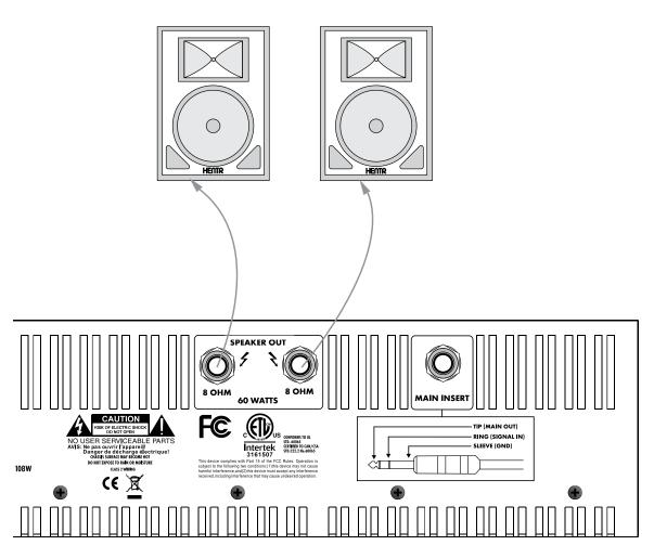
CAUTION: Minimum 4  $\Omega$  load. Use a maximum of two 8  $\Omega$  speakers.
