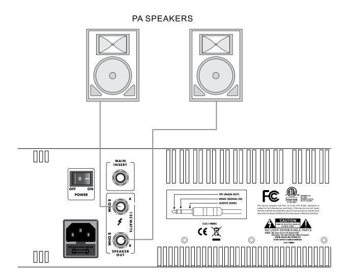
CAUTION: Minimum 4 $\Omega$  load. Use a maximum of two 8 $\Omega$  speakers.
